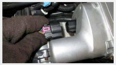
Disconnect the electrical connector at the throttle body. Remove the four 10mm bolts that secure the throttle body to the intake manifold and place it on a workbench.
