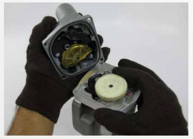
Using the supplied special Torx T-25 bit remove the four bolts that secure the throttle body motor to the throttle body. Remove the motor by gently lifting up. Also remove the white gear by sliding it up off the pin. Transfer the gear and motor to the BBK Throttle Body and tighten the motor with the stock hardware.
