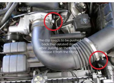
Loosen the clamps at the throttle body and factory air box.
