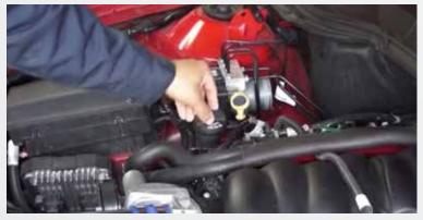
Remove the oil cap and the decorative engine cover by gently pulling up to pop it off the rubber mounts. Replace the oil cap to prevent debris from contaminating the oil.
